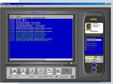
All operator actions and system transactions are automatically logged to the hard disk and can be viewed, printed, emailed or exported to provide detailed reports of events.
